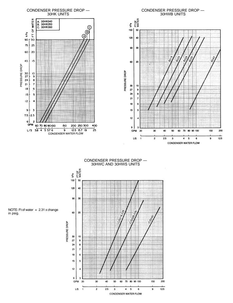
Fig. 16 — Cooler and Condenser Water Pressure Drop (cont)
